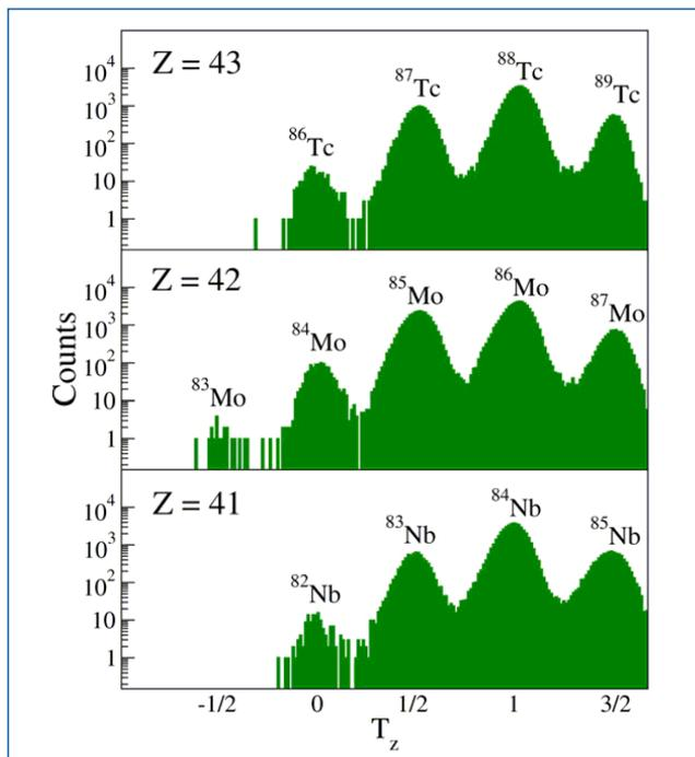
Fig. 6. Projections of the particle identification spectra from the fragmentation of a  $^{107}\text{Ag}$  primary beam to populate isomeric states in the odd-odd  $N=Z$  proton drip-line nuclei  $^{82}\text{Nb}$  and  $^{86}\text{Tc}$ .
