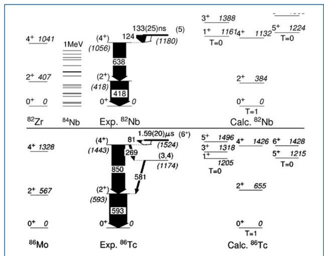
Fig. 8. Comparison of projected shell model calculations including  $T=0$  and  $T=1$  pairing for  $^{82}\text{Nb}$  and  $^{86}\text{Tc}$  with the experimental results from RISING.
