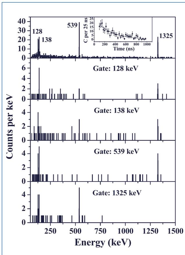
Fig. 11. Stopped RISING gamma-ray spectra showing the decay of the proposed spin/parity  $8^+$  in the 2-proton hole, r-process path nucleus,  $^{130}\text{Cd}$ .
