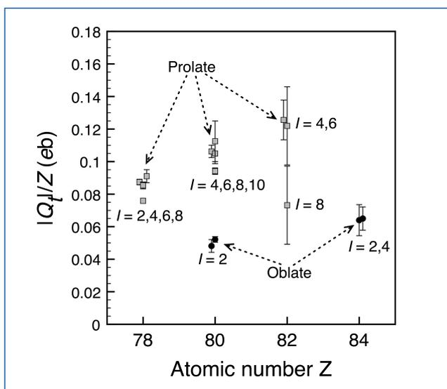
Figure 11. Experimental transition quadrupole moments normalised by the atomic number  $Z$  for the transitions between prolate (grey squares) and oblate (black circles) states in  $^{182}\text{Pt}$ ,  $^{182}\text{Hg}$ ,  $^{186}\text{Pb}$  and  $^{194}\text{Po}$  nuclei in the vicinity of the neutron mid shell. The initial spin  $I$  ranges for the selected states are indicated.
