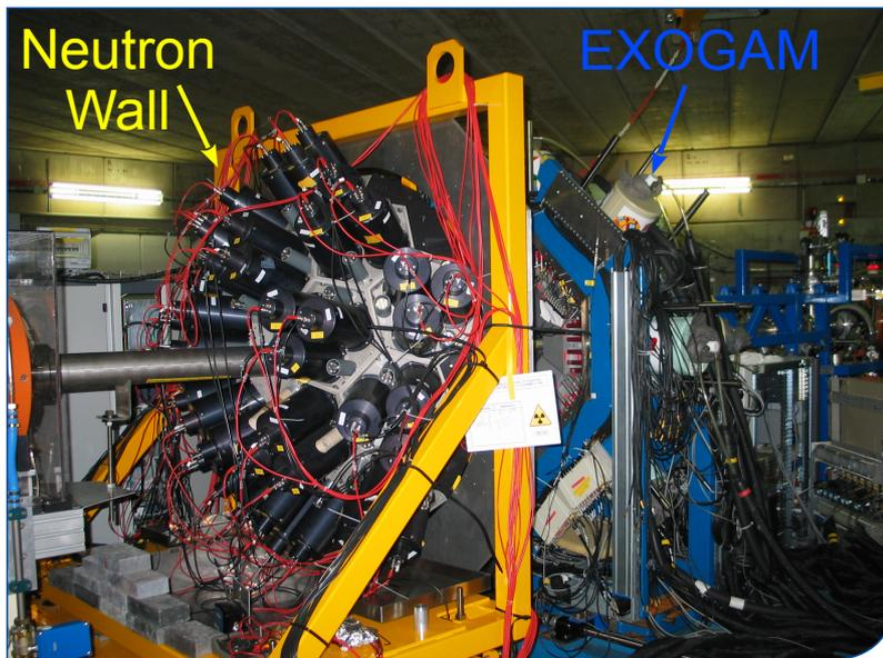
Fig. 1. Neutron Wall and EXOGAM at GANIL.
