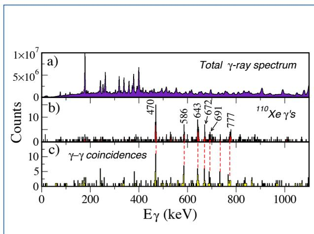
Fig. 9. (a) Total  $\gamma$ -ray spectrum correlated with any fusion-evaporation channel open in the experiment. (b)  $\gamma$  rays identified in  $^{110}\text{Xe}$  by means of ‘mother-daughter’ alpha-decay tagging. (c) A  $\gamma$ - $\gamma$  coincidence spectrum from a sum of gates on the strongest transitions. The staggering selectivity allows access to excited states in  $^{110}\text{Xe}$  at a  $\sim 50$  nb reaction cross-section.
