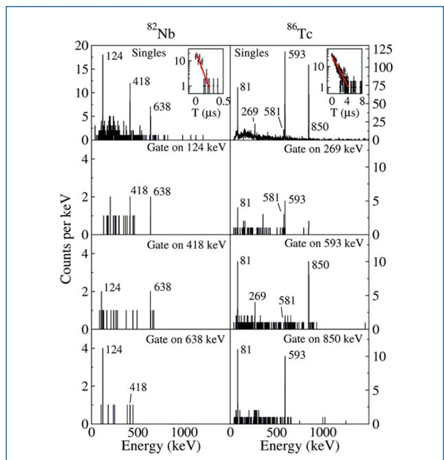
Fig. 7. Stopped RISING gamma-ray spectra showing the decays of the isomeric states in  $^{82}\text{Nb}$  and  $^{86}\text{Tc}$ , including gamma-gamma coincidence spectra between these transitions.
