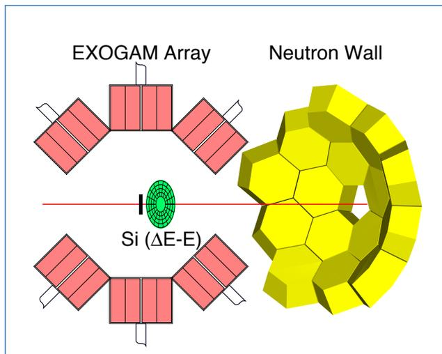
Fig. 5. Experimental setup in the  ${}^6,8\text{He}+{}^{65}\text{Cu}$  experiments. [A. Chatterjee et al., Phys. Rev. Lett. 101 (2008) 032701].
