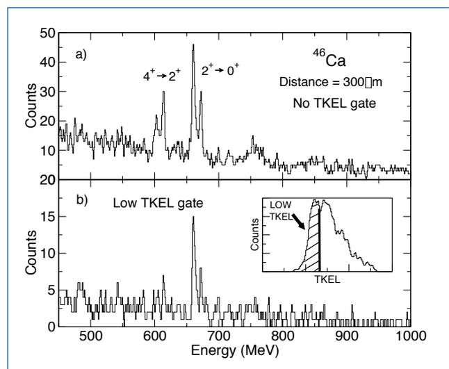
Fig. 7: Doppler-corrected  $\gamma$ -ray spectra corresponding to the  $2^+ \rightarrow 0^+$  1346 keV and  $4^+ \rightarrow 2^+$  1229-keV transitions in  $^{46}\text{Ca}$  for different TKEL cuts, a) gate on low TKEL and b) gate on high TKEL.
