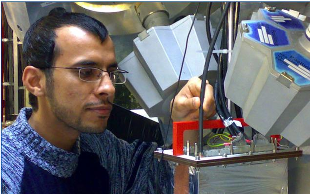
Fig. 14. The Stopped RISING ‘active stopper’ which allowed beta-delayed gamma-ray coincidence measurements to be performed in a range of exotic nuclei.
