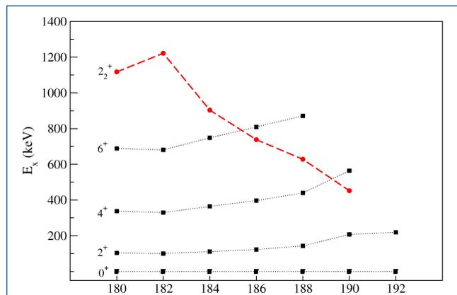
Fig. 17. Excitation systematics of W isotopes following the additional data for states in  $^{190,192}\text{W}$  from the Stopped RISING Campaign. The evolution of the first and second  $2^+$  states is consistent with the predicted evolution towards a triaxially, gamma-soft nuclear ground state shape around  $N\sim 114-116$ .
