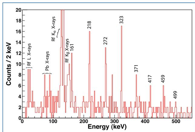
Fig 2. Fission-tagged gamma-ray singles spectrum of  $^{256}\text{Rf}$
