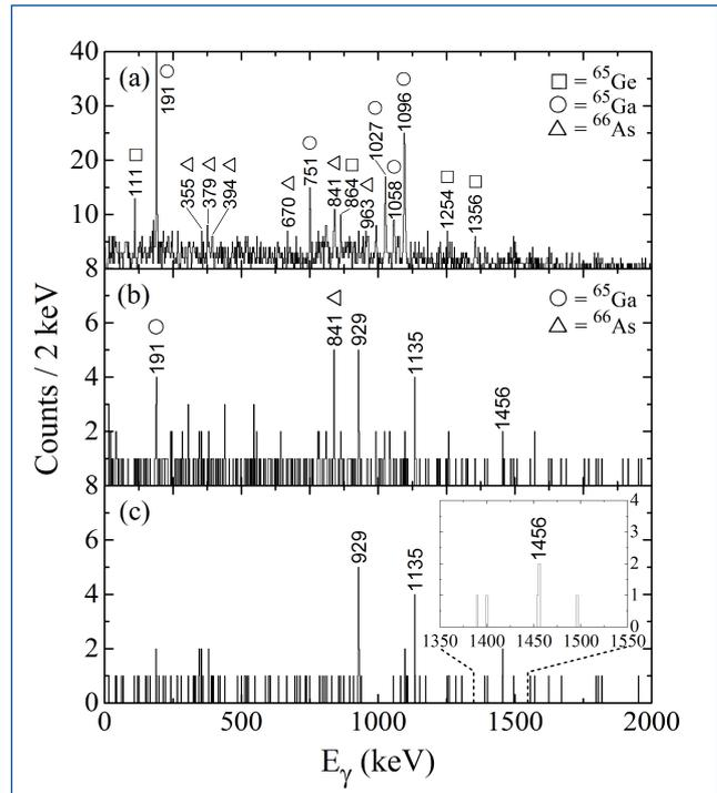
Fig. 7. (a) Recoil- $\beta$  tagged JUROGAM II singles  $\gamma$ -ray spectrum. (b) Same as (a) but with charged-particle suppression. (c) Same as (b) but with an additional delayed  $\gamma$ -ray veto condition.
