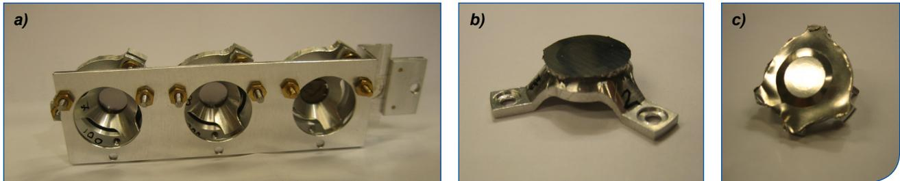
Fig. 5. a) A ladder holding three different target-to-degrader distances, b) the target and c) the degrader.
