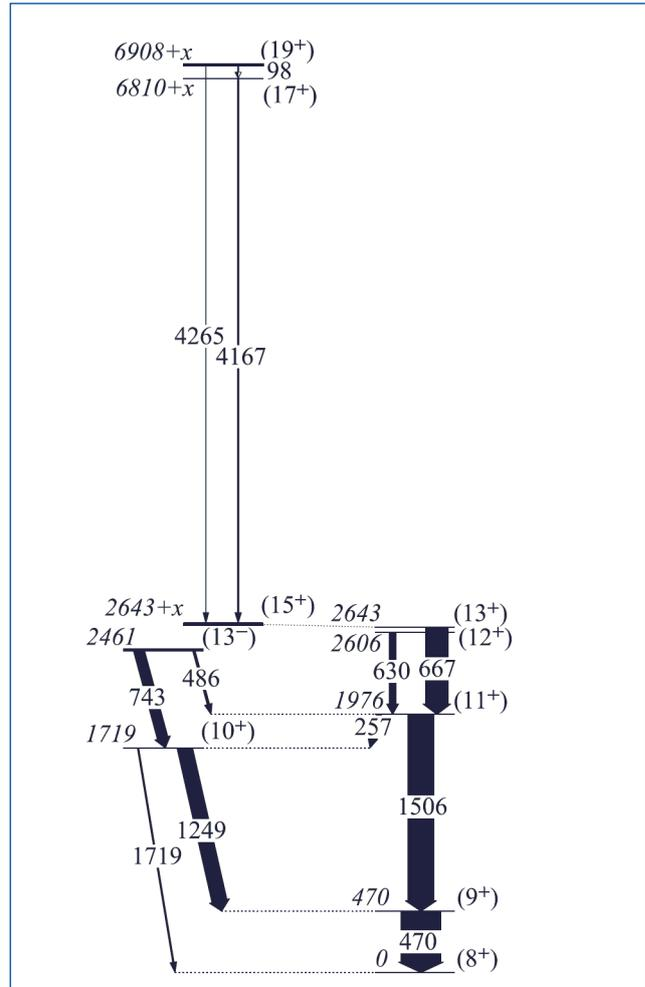
Fig. 10. Proposed level scheme of  $^{96}\text{Ag}$ . The isomeric states identified in this experiment are drawn in bold.
