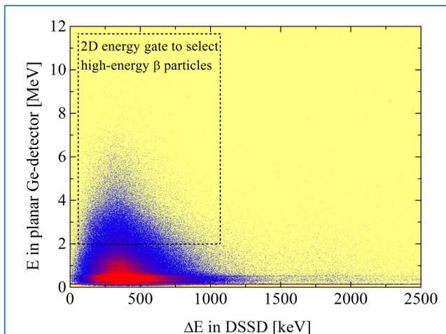
Fig. 6. Identification of high-energy  $\beta$  particles from a  $\Delta E$ - $E$  spectrum of the focal-plane DSSD and planar Ge-detector.
