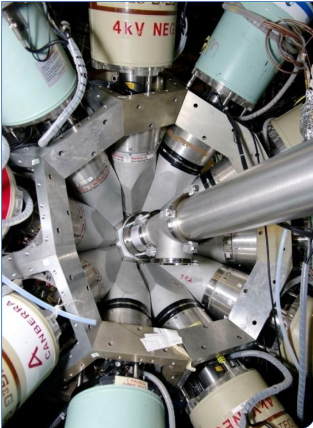
The Orsay Gamma Array (ORGAM) has been installed and running at IPN Orsay/France since 2009. It is dedicated to gamma ray spectroscopy using stable beams accelerated by a 15 MV MP-Tandem Accelerator.
