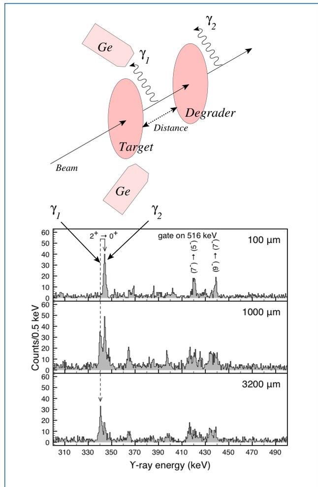
Figure 12. The principle of the RDDS technique with degrader foil.
