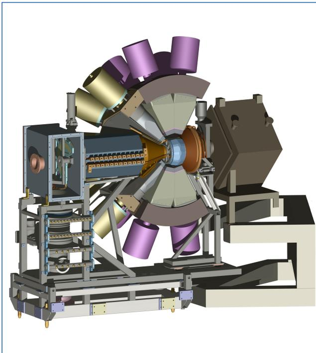
Fig. 13. Schematic design of the SAGE spectrometer coupled to RITU. [J.Pakarinen et al., EPJA (2014) 50: 53]
