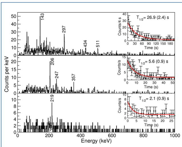
Fig. 15. Beta-delayed, Stopped RISING gamma-ray spectra showing the decays of  $^{188,190,192}\text{Ta}$  into excited state of  $^{188,190,192}\text{W}$ .
