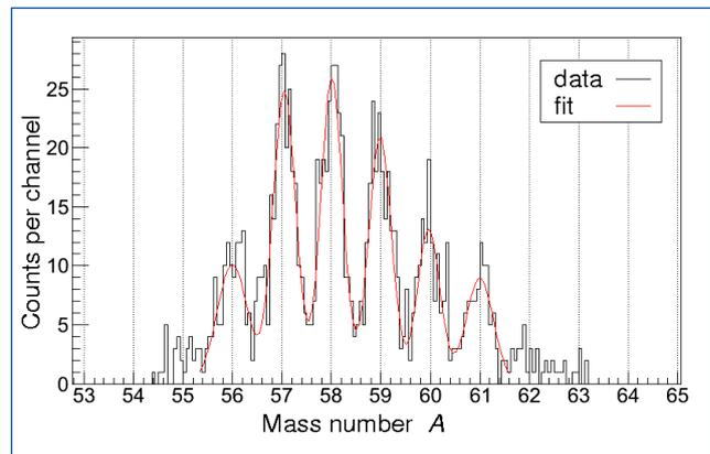
Fig. 1: LYCCA mass-identification plot for Fe fragments [P. Golubev et al., Nucl. Instr. Meth. A723, 55 (2013)].
