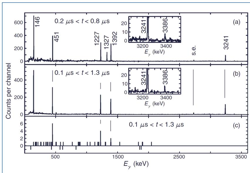
Fig. 3. Stopped RISING gamma-ray spectra showing the decay of the  $^{54}\text{Ni}$   $10^+$  isomeric state.
