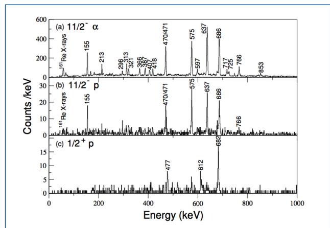
Figure 16. Gamma rays selected by recoil-decay correlations with the alpha and proton decays from the  $1/2^+$  and  $11/2^-$  states in the proton emitter,  $^{161}\text{Re}$  [K. Lagergren et al., *Phys. Rev. C* 74, 024316 (2006)].
