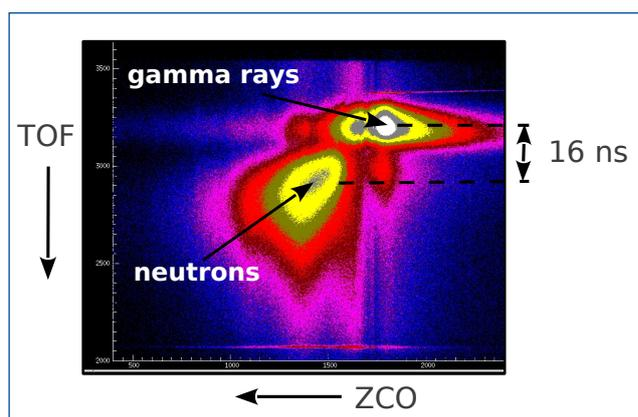
Fig. 3. Zero-Crossover Time (ZCO) versus Time-of-Flight (TOF) measured by one of the Neutron Wall detectors.
