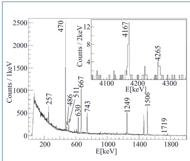
Fig. 9. A  $\gamma$ -ray spectrum observed with RISING from 0.075 to 90  $\mu\text{s}$  after implantation of  $^{96}\text{Ag}$ . The inset highlights the region around 4 MeV.
