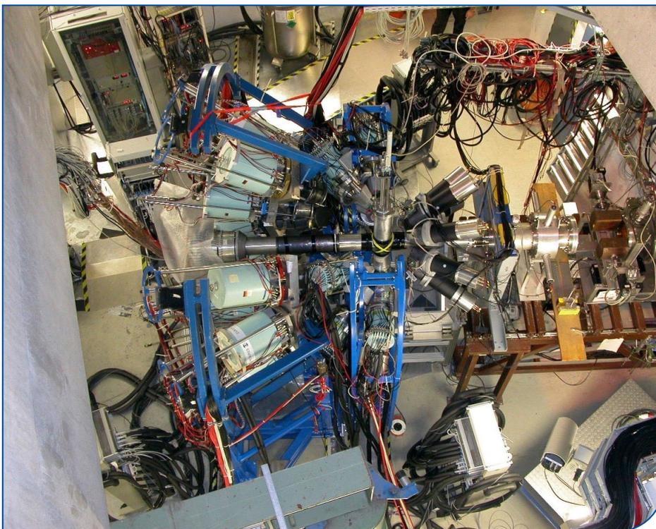
Fig. 1: RISING in-beam set-up. The beam enters the set-up from the right. After hitting the target the ions are detected in the CATE detector. The  $\gamma$ -rays are detected using the HECTOR array (right), the MINI-BALL detectors (middle) and the EURO-BALL Cluster detectors (left).
