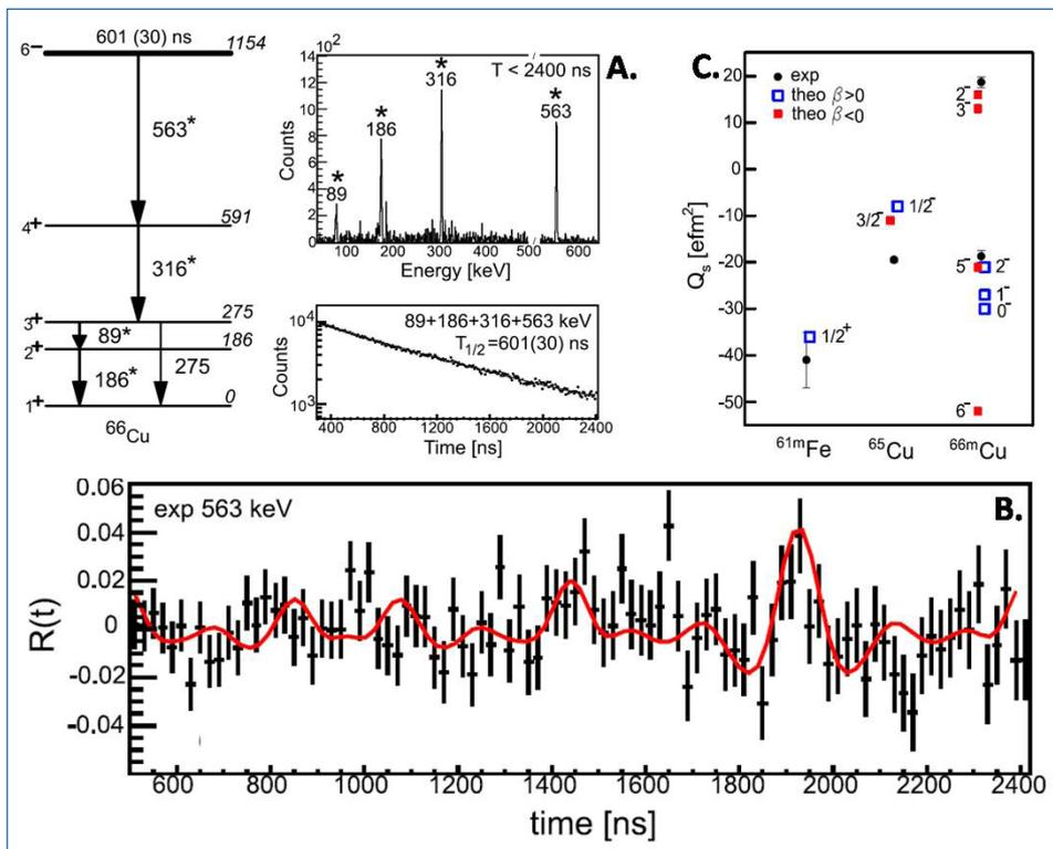
A. Decay scheme of the 6<sup>-</sup> isomer in <sup>66</sup>Cu along with the delayed background subtracted gamma and time spectra; B. R(t) function for the 563 keV (M2) transition; C. Experimental Q<sub>s</sub> for <sup>61m</sup>Fe(9/2<sup>+</sup>), <sup>65</sup>Cu(3/2<sup>-</sup>) and <sup>66m</sup>Cu(6<sup>-</sup>) (full circles) are compared to the theory for oblate (full squares) and prolate (empty squares) shapes. The theoretical predictions are labeled with their K<sup>π</sup> value.
