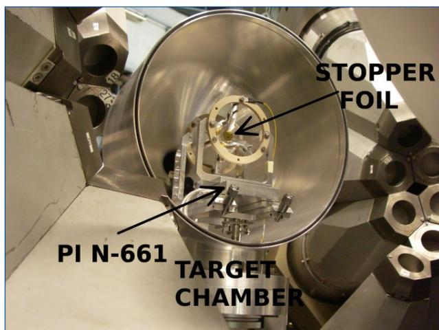
The OUPS Plunger inserted in the reaction chamber of ORGAM.
