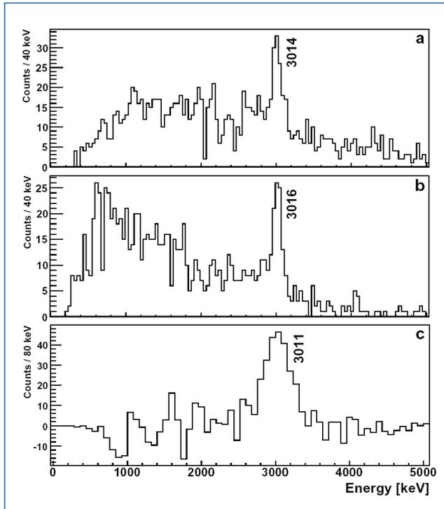
Fig. 3: Doppler corrected  $^{36}\text{Ca}$  gated  $\gamma$ -ray spectra measured with the Cluster (a), MINIBALL (b) and HECTOR (c) detectors. For (c) the background was subtracted.
