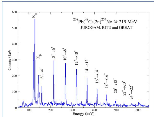
Fig1. Recoil-gated spectrum of  $\gamma$ -rays from  $^{254}\text{No}$
