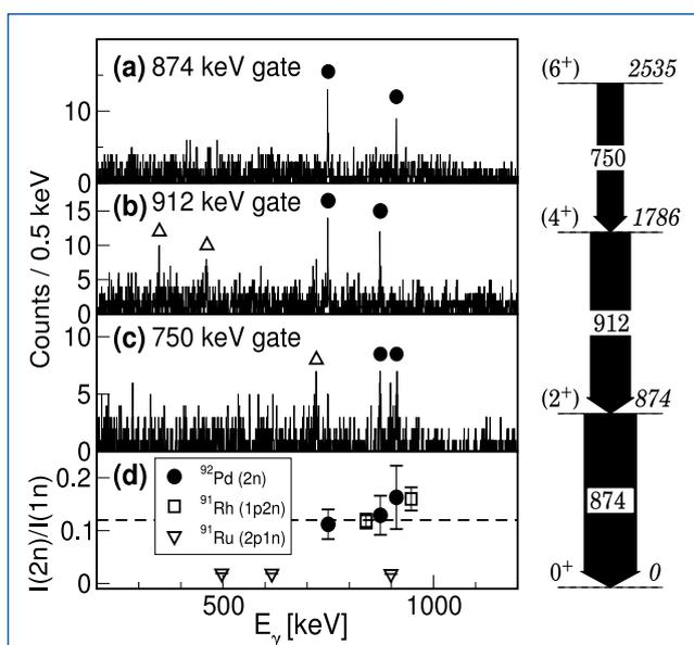
Fig. 2. Identification of  $\gamma$ -ray transitions in  $^{92}\text{Pd}$ . The  $\gamma$  rays are in coincidence with two neutrons but not in coincidence with any charged particles. [B. Cederwall et al., Nature 469 (2011) 68].
