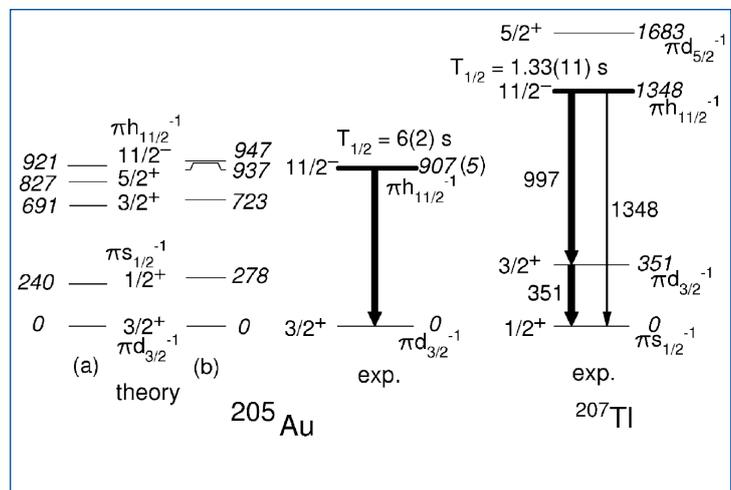
Figure 18: Calculated and experimental level schemes of  $^{205}\text{Au}$ . For comparison the partial level scheme of  $^{207}\text{Tl}$  is also given.
