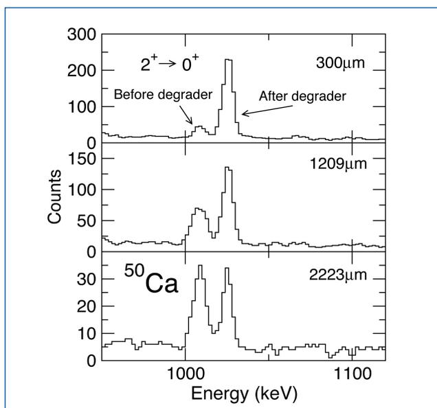
Fig. 6: Doppler-corrected  $\gamma$ -ray spectra showing the  $2^+ \rightarrow 0^+$  1027-keV and transitions in  $^{50}\text{Ca}$  for different target-to-degrader distances. The higher-energy and lower-energy peaks correspond to the decays after and before the degrader, respectively.
