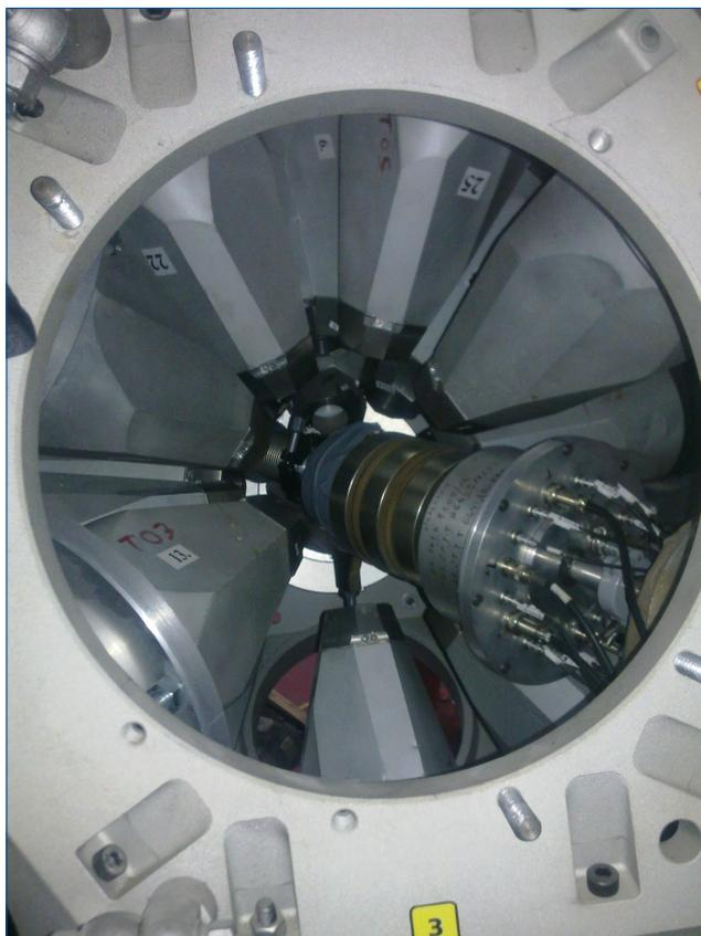
Fig.1 The EAGLE array of 15 HPGe Gammapool detectors coupled to the electron spectrometer [J. Andrzejewski et al., *Nucl. Inst. and Meth. A* 585 (2008) 155] for electron-gamma and gamma-gamma coincidence measurements.
